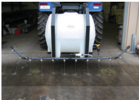
225 gal. skid mounted
