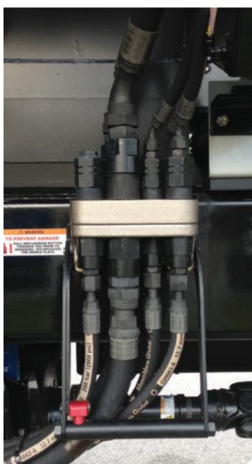
Quick disconnect for faster change-overs, featuring corrosion resistant fittings and hardware.
