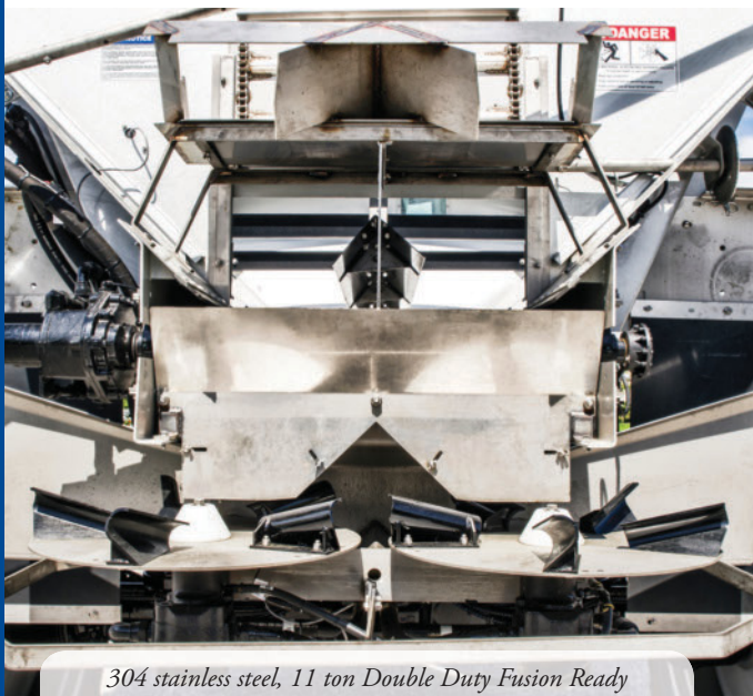
11 ton Double Duty Fusion Ready spreader with floatier tires
